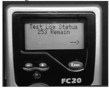
om ' From this window, pressing Function takes you to the Battery Status display. Pressing Exec. while in the Test Log Status window takes you to this display:
