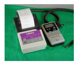
Connect the printer cable with the notches facing forward and the screws facing up. Attempting to force a connection with a printer cable in the wrong position may damage the instrument.
