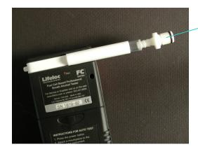
This fitting should be inserted farther into the clear tubing. It is this way for display purposes only.
