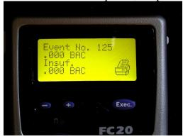
To print this test, press **Exec.** If the printer is not currently attached, the test may be printed later. Except for performance verification checks (Wet Checks) see page 21.
