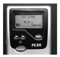
rensic services To get a more accurate indication of battery condition, press Function repeatedly until the **Status** window appears, then press **Exec./Function/Function** to see the actual battery voltage. At 4.4 volts the instrument will no longer operate and the display will show "Warning Low Battery". Replace with fresh alkaline batteries.
